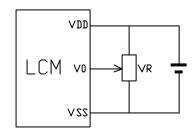
$V_{DD\sim}V_0$ : LCD Driving voltage
